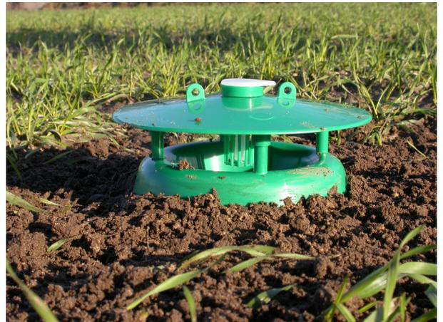
Bury trap into the soil so that the trap funnel is just above the soil surface.
